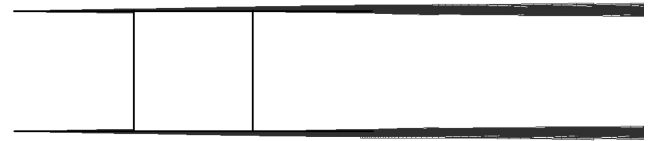
Fig. 5 Boundary-layer region selected for computation of the nacelle drag in flat nacelle test, M_{\infty} = 0.5 , \alpha = 0 deg, and Re_l = 1 \times 10^6 , power-off condition.
